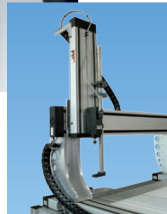
→ Extra high passage (here 500 mm) with long z axis.
