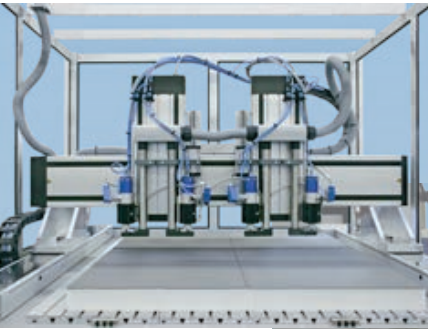
→ Detail view of the front clamping range of a CAM 1010 Premium – very practical for working on housings etc.
